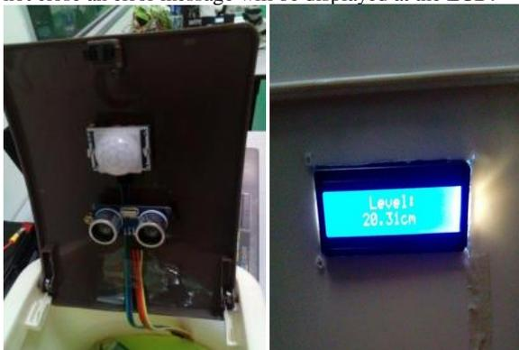
Fig. 7: Sensors attached at the waste bin lid.
