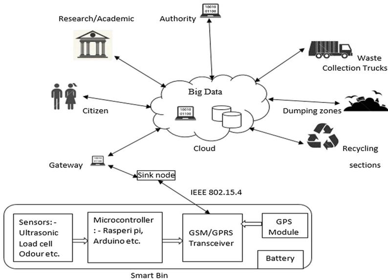
Fig. 3. The proposed framework for smart bin system.
