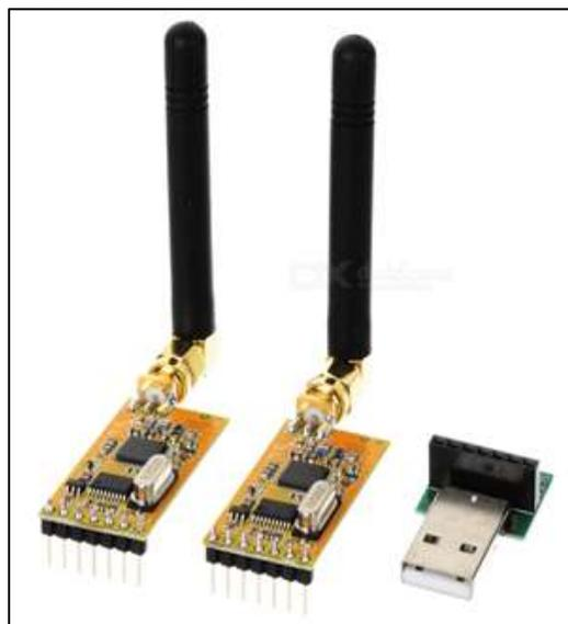
Fig. 4: RF transmitter and Receiver module
