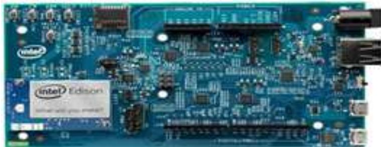
Fig. 1: Intel Edison Development Board for Arduino
