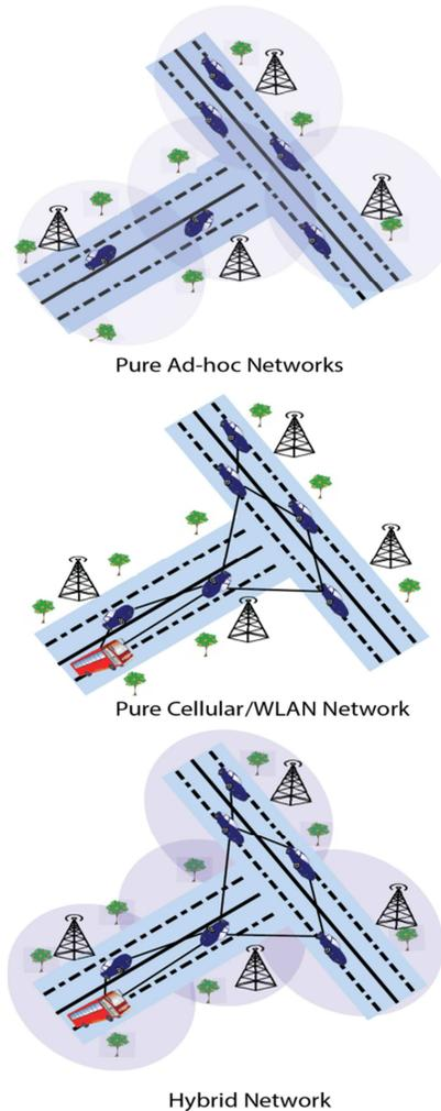
Fig 1. Three Architectures of VANET Pure Ad-hoc Networks, Pure Cellular /WLAN Networks, Hybrid Architecture
