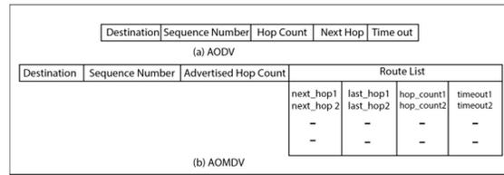
Fig 3. Entry Structure of routing table (a) AODV (b) AOMDV
